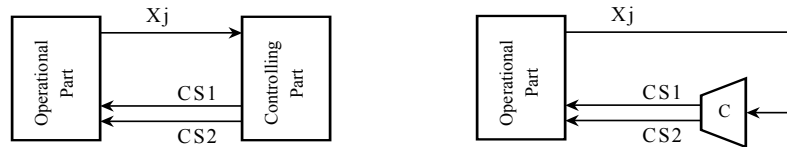
Fig. 10 Removing the controlling automata
